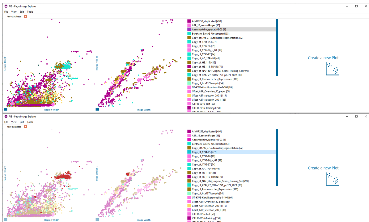
Figure 1: UI of PIE showing all documents with different features selected. The bottom screenshots shows the selection of a document. It can be seen that it's pages are clustered in the feature space (red dots).
