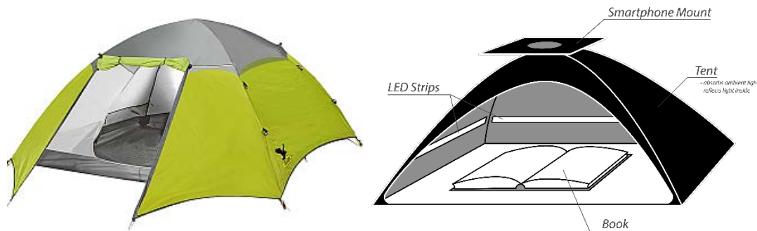
Figure 1 Typical “dome tent” with its characteristic form (here from the Italian company Salewa) and a sketch of the planned ScanTent
