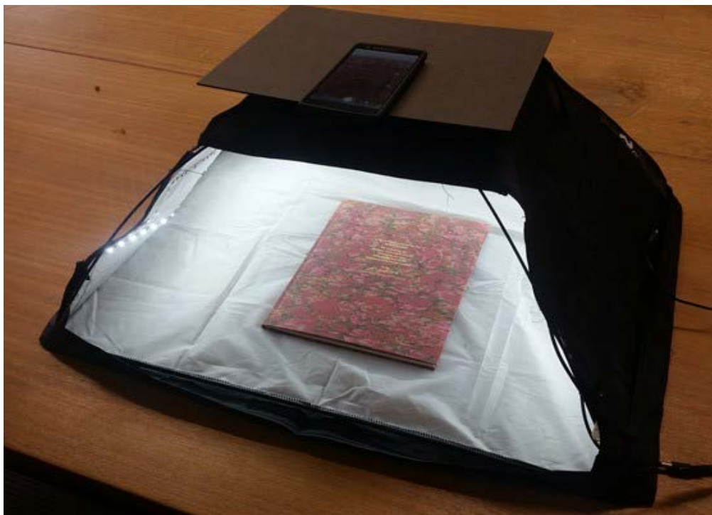
- Figure 3 ScanTent - prototype – lights turned on
