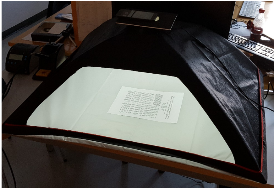
Figure 5: ScanTent – prototype with 3D plotted mount for the smartphone
